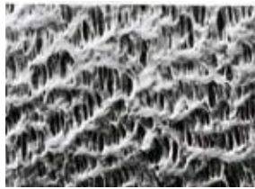
Magnified view of the hollow fiber membrane surface
