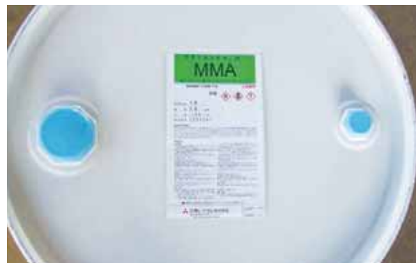
A GHS compliance label is affixed to the top of a drum containing MMA monomers.
