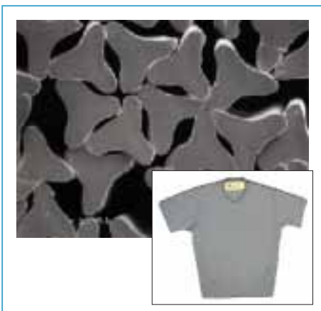
ECORNA-Y Cross-section and Jersey
